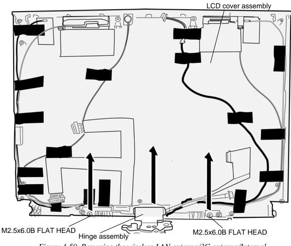
Figure 4-59 Removing the wireless LAN antenna/3G antenna/Internal microphone/webcamera cable(3G model only)
